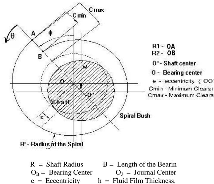
**Figure - 1: Physical configuration of Convergent Spiral Squeeze film Bearing..**
