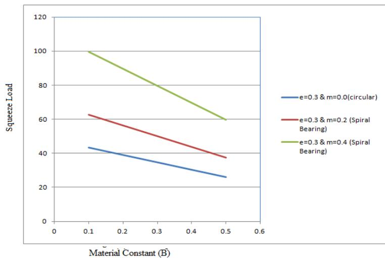
Figure-3: Squeeze Load vs Material Constant at constant Eccentricity ratio for both Circular and Spiral Bearings.
