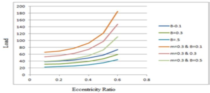
Figure-2: Squeeze load vs Eccentricity ratio at different Material Constant and Preload factor.
