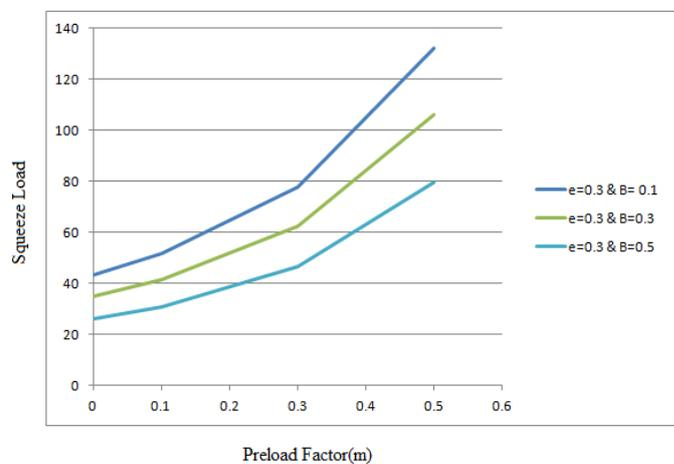
Figure-4: Squeeze Load vs Preload Factor(m) at constant Eccentricity Ratio for different Material Constant.
